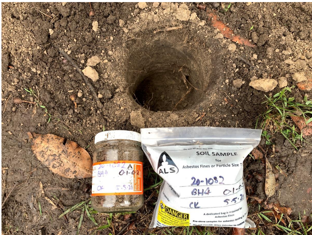
Photo 15: Showing borehole BH4 sampling location at 10 Marshall Avenue, St Leonards.
